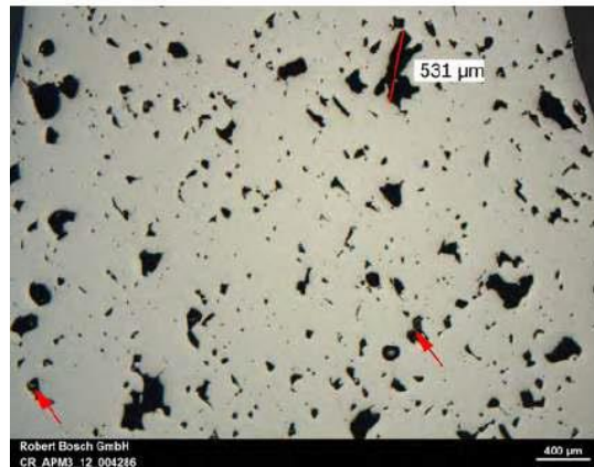
Figure 6- Microscopic image showing pores formed due to insufficient energy.
