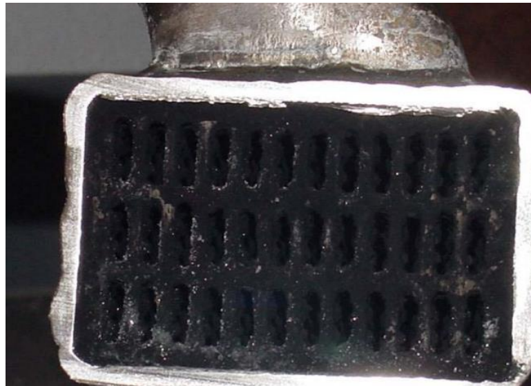
Figure 1.2 – Image of a fouled EGR heat exchanger. 15
