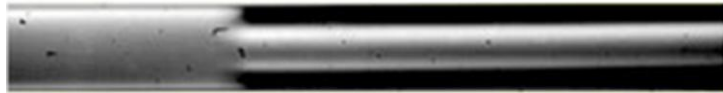
Figure B.2. Time lapse image of displacement of gas showing clean displacement showing a distinct gas-liquid interface (Moore, 2012).
