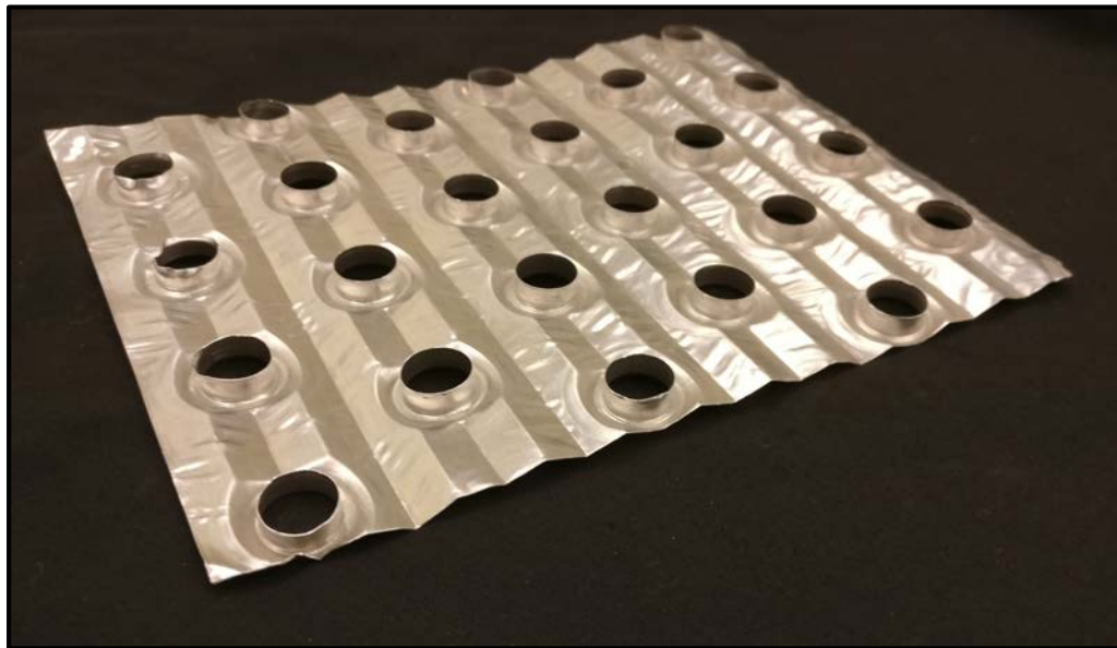
Figure 6.2 Sample corrugated-fin with collars
