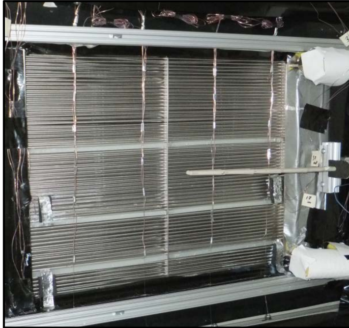
Figure 4.13 Photograph of Condenser M.1 with the outlet thermocouple array
