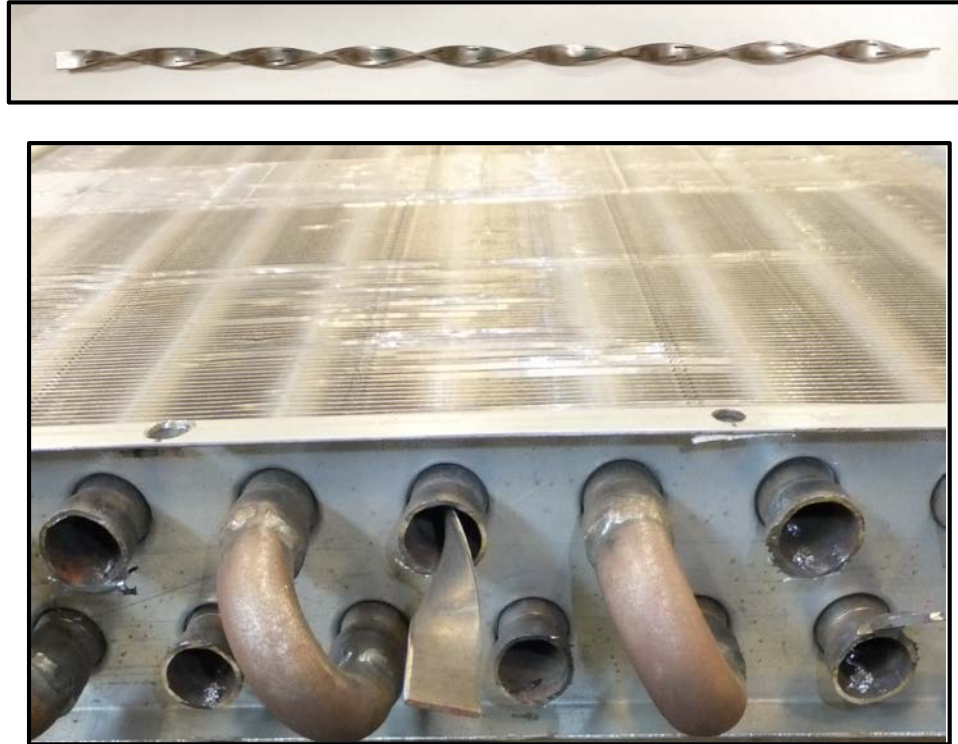
Figure 6.1 Twisted tape (top) and twisted tape being inserted into round-tube corrugated-fin condenser (bottom)
