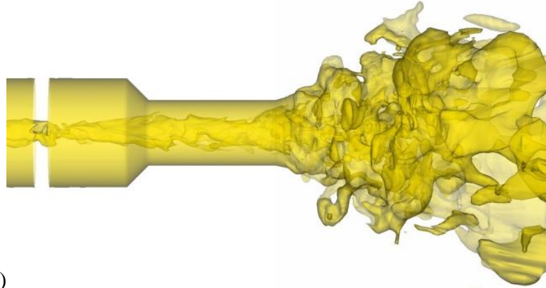
Figure 4.7: (a) Instantaneous distribution of density field with two iso-surfaces: \rho = 532 and 250 \text{ kg/m}^3 ; (b) iso-surface of azimuthal velocity at u_0 = 4 \text{ m/s} ; p=100 \text{ atm}
