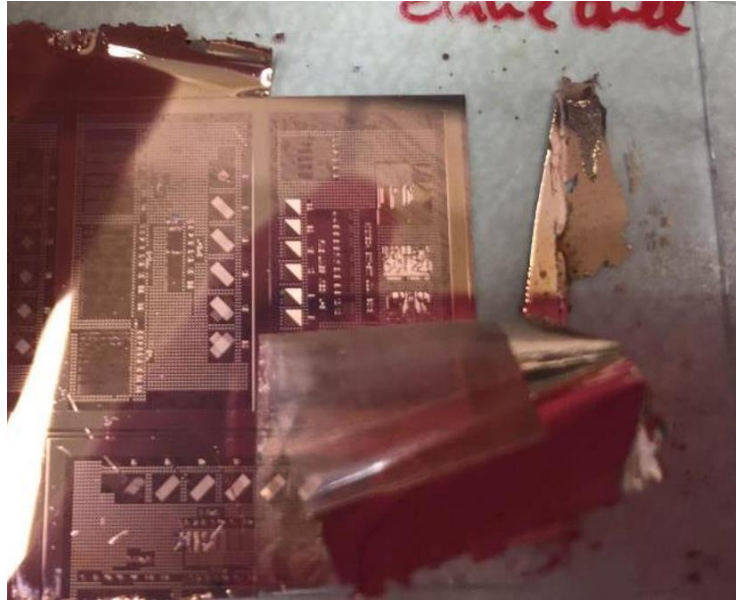
Figure 7 – Copper peeling from bare glass (credit: Bernhard).
