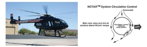
Figure 2.10. MD600 that utilizes the NOTAR system on the tail boom (left) and cross sectional view of the tail boom (right) (Stephens 2012)
