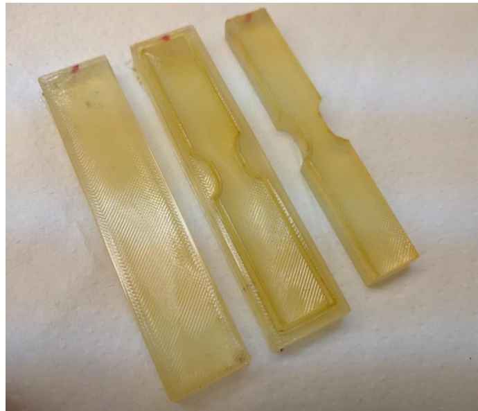
Figure 6.1: Image showing printed sheet stock, laser cut sheet, and final sample.
