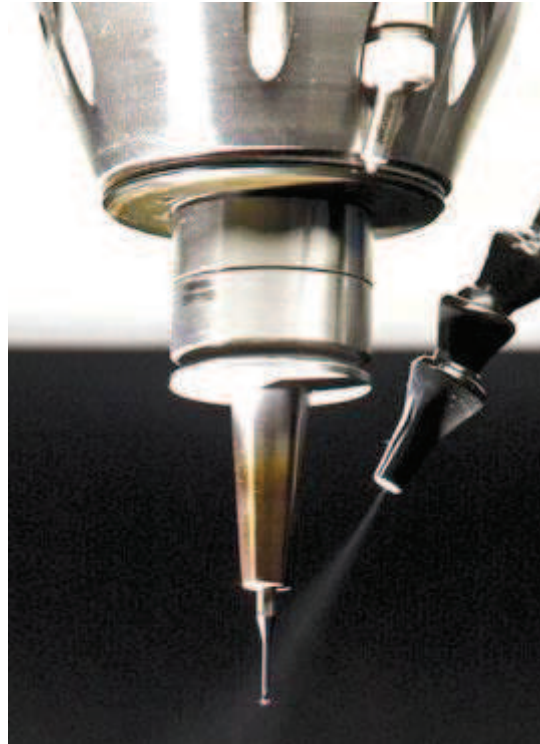
Figure 2.6: MQL cooling of a micro end mill (Modern Machine Shop).
