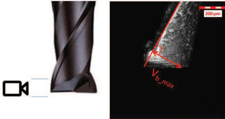
Figure 5.17: Peripheral flank wear measurement example.
