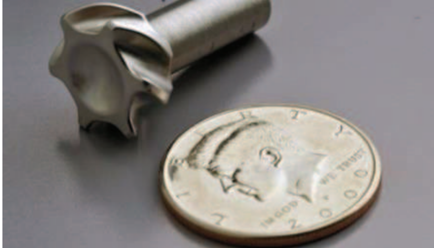
Figure 1.2: Fluid impeller part, machined in a 5-axis micro mill (Microolution Inc.).
