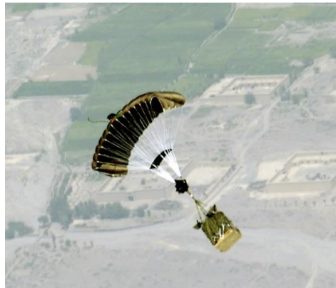
Figure 1.1: The guided PADS being controlled during its descent (Image credit: http://www.defenseindustrydaily.com/jpads-making-precision-airdrop-a-reality-0678/ )
