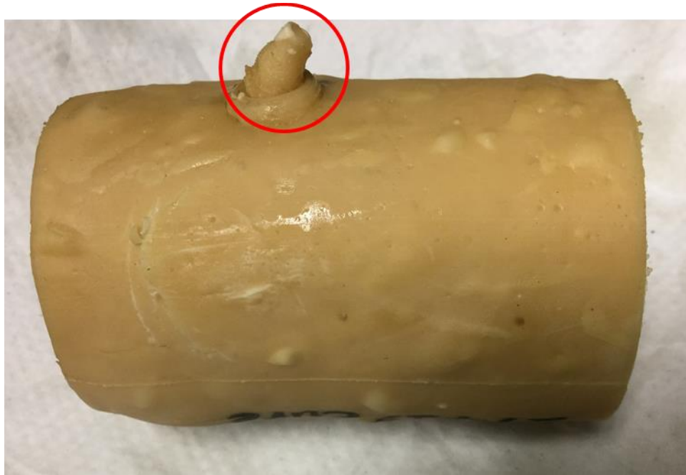
Figure D-1: Damaged Vytaflex Foam after high pressure and temperature, port extrusion circled
