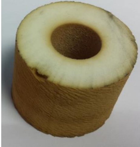
Figure 4-14: First generation foam stained by oil
