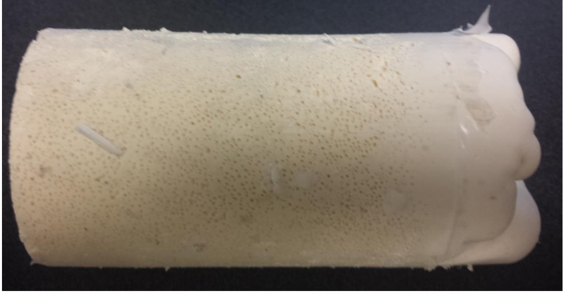
Figure D-8: Sylgard 184 foam with burst microspheres
