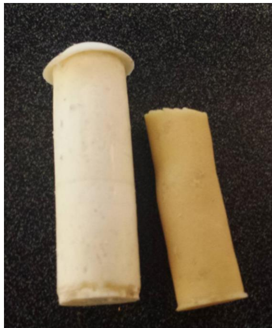
Figure D-3: Undamaged plug (left) damaged Vytaflex plug (right)
