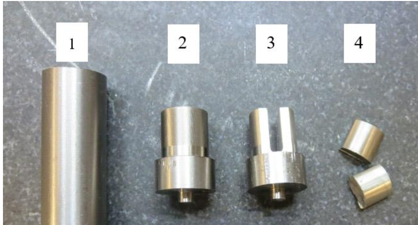
Figure 19: In vitro sample manufacturing procedure. (1) turn cylindrical stock to specified diameter, (2) texture rod (if using MAT process) and part from stock, (3) use end mill to face and slot part, (4) use wire EDM to cut two curved samples from each workpiece.
