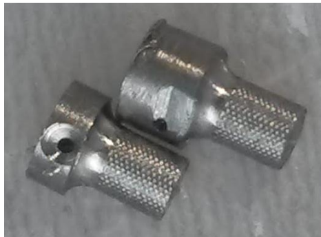
Figure 23: Representative test samples used in in vivo testing. Top right sample does not have the final side milling step, which shortens the implant to the sample seen on the bottom left
