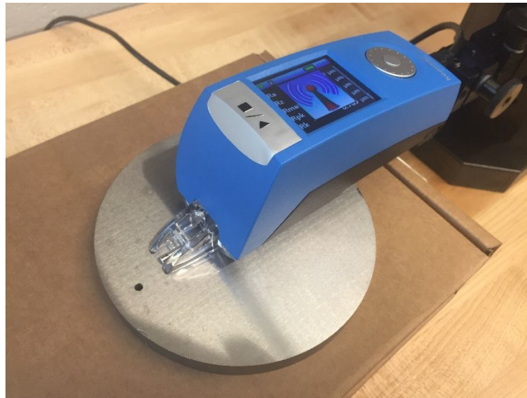
Fig. 2.41 Stylus profilometer used to measure the surface roughness.
