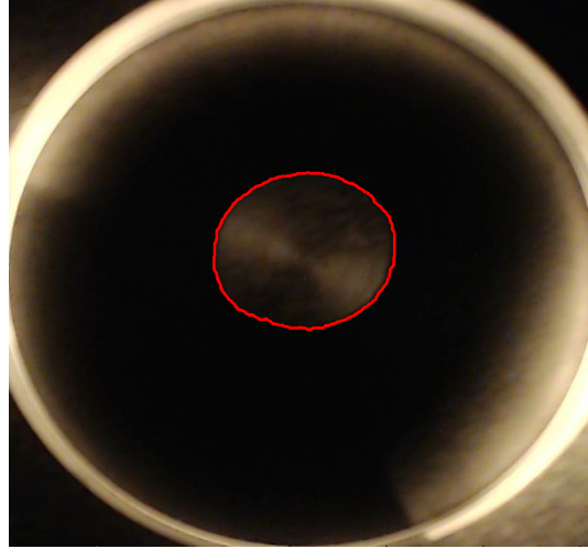
Fig. 2.58 Measured wetted area between two contacting surfaces.
