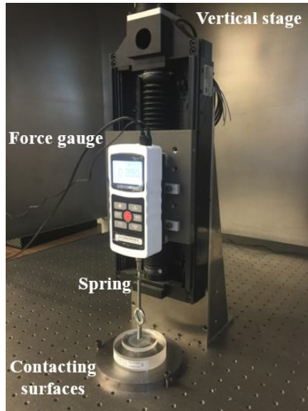
Fig. 2.40 Experimental setup to measure the pull-off force.
