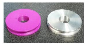
Figure 2. Printed and Machined Pulleys
