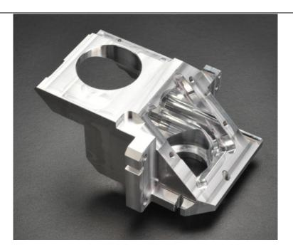
Figure 43. Multi-Setup Milled Part for PQ 8
