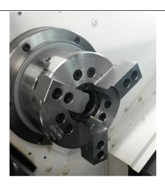
Figure 11. Softjaws for Yoyo Machining
