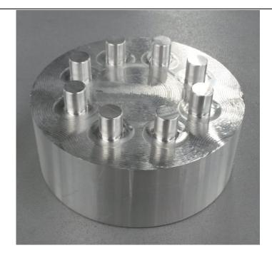
Figure 13. Alignment Rig for Millturn Machine
