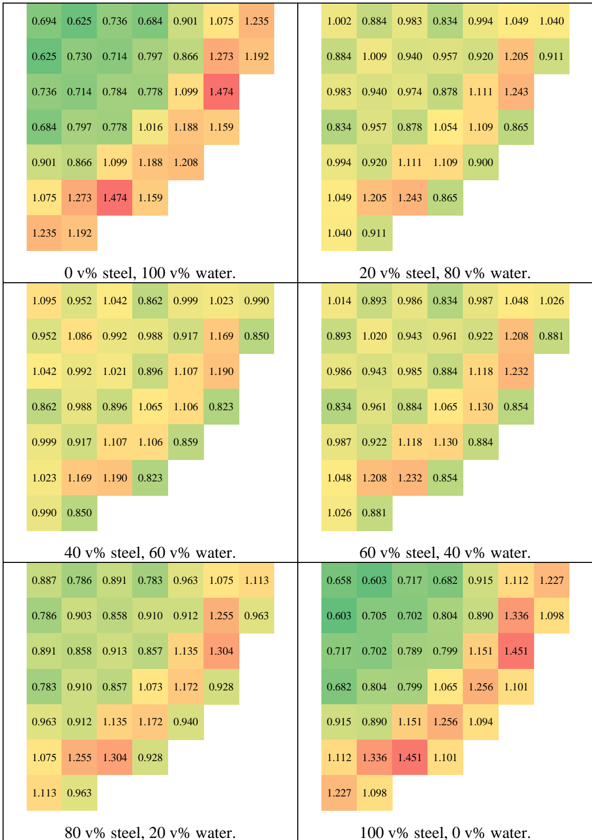
Figure 4.22 Radial profiles for 0 ppm boron with varying radial reflector compositions.
