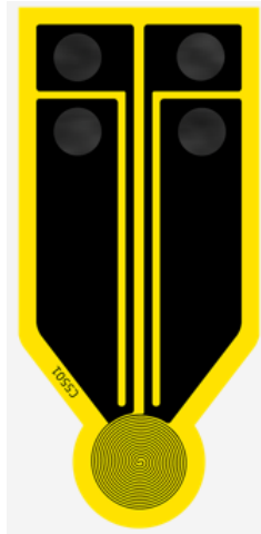
Figure 3.11 Kapton-insulated Hot Disk sensor [41]
