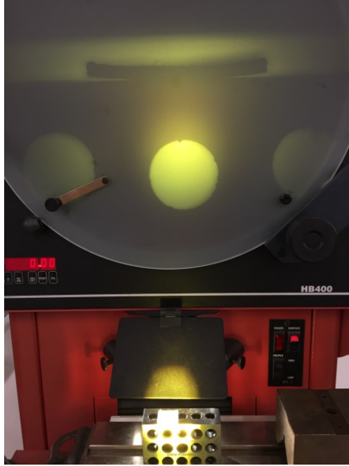
Figure 4.29 Part warpage measurement using an optical comparator
