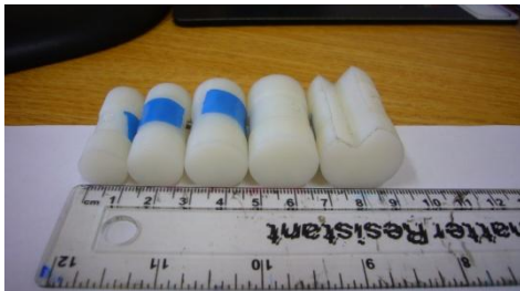
Fig. 7.3 The cylindrical rods used to estimate the bending radius of curvature of the device.
