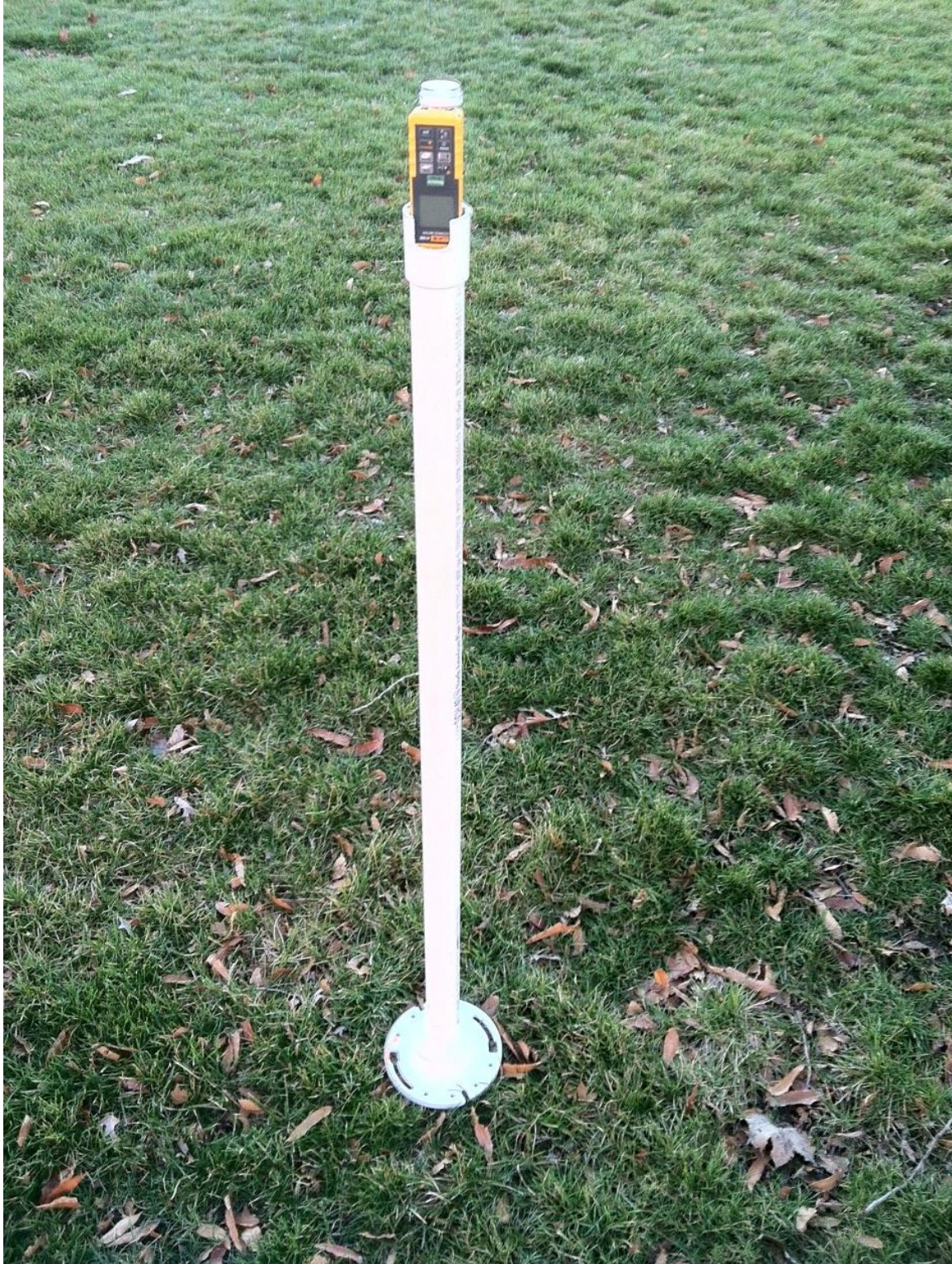
Figure 4.3 - Fluke® 416D laser distance meter mounted on purpose-built measurement stand.
