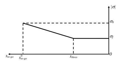
Figure 4.1 Bank angle parametrization with respect to range-to-go  $s_{to-go}$
