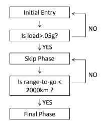
Figure 4.2 Phase transition logic for planning
