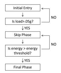
Figure 4.8 Phase transition logic with energy (discontinuous planning)
