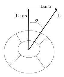
Figure 2.2 Modulation of bank angle by rolling
