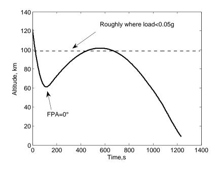
Figure 4.6 Discontinuous planning: time versus altitude-first iteration
