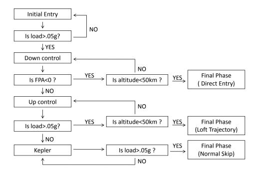
Figure 4.4 Phase transition logic with discontinuous planning
