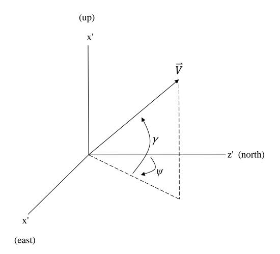
Figure 6.2 Velocity LVLH coordinate system
