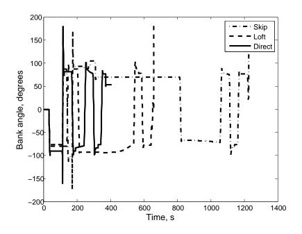
Figure 5.3 Bank angle histories for different trajectory types
