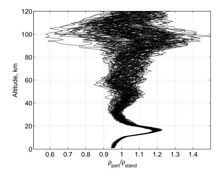
Figure 6.4 Ratio of GRAM 07 perturbed atmosphere to US 76 standard atmosphere as a function of altitude for 100 cases.
