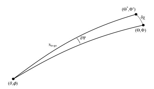
Figure 5.4 Crossrange biasing diagram
