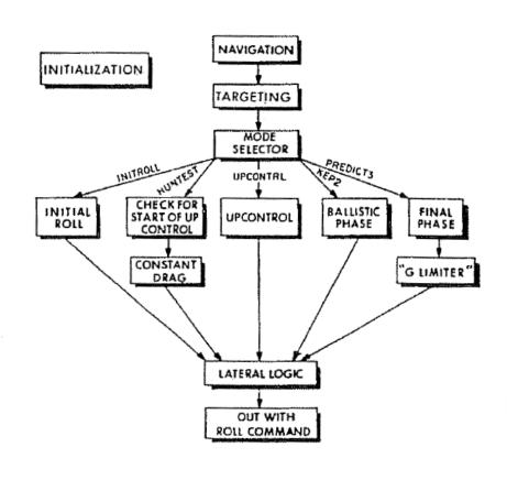
Figure 3.1 Guidance flowchart for Apollo skip algorithm[4].
