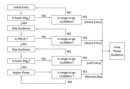
Figure 5.1 Phase transition logic for guidance
