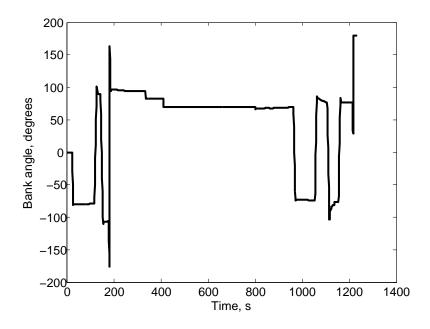
Figure 7.2 Bank angle profile for the nominal northbound medium range case (8400km).
