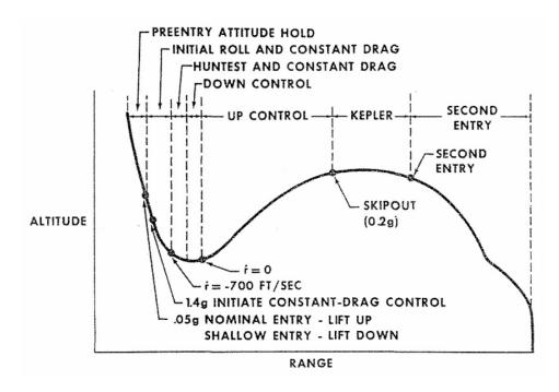
Figure 3.2 Reentry guidance phases for Apollo skip algorithm[5].
