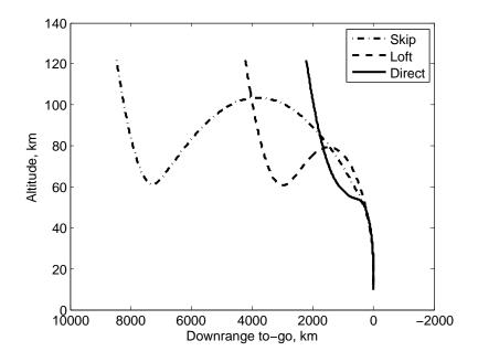
Figure 5.2 Possible entry trajectory types
