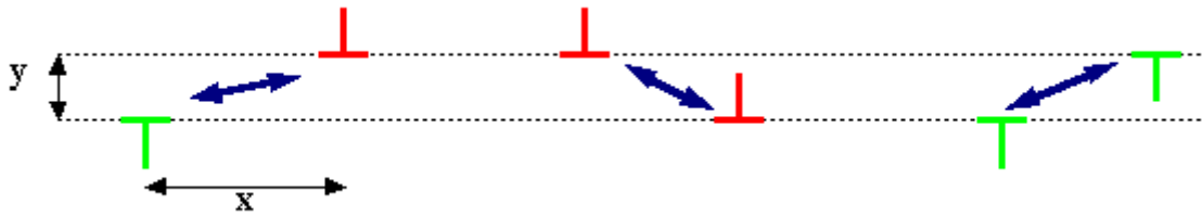
Figure 4.9 Edge dislocations with identical or opposite Burger's vector \underline{b} on neighboring glide planes
