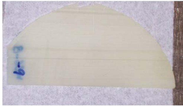
Fig. 1.8 Optical image shows the surface waviness, roughness, chipping
