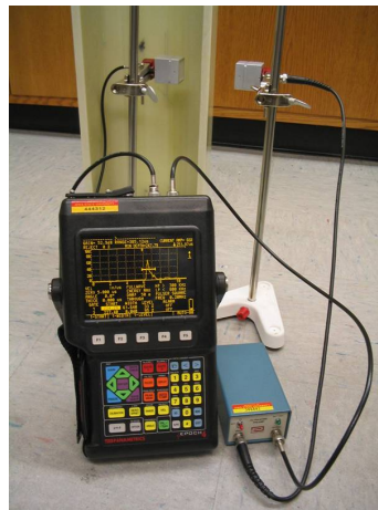
Figure 4.3 The Panametrics Epoch 4 shown with the Ultran GMP transducers performing an A-Scan through GS1.
