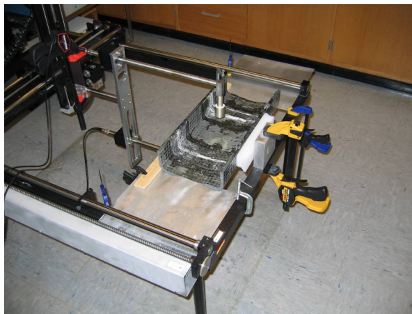
Figure 5.14 The scanning setup used for the CS1 wing spar section.
