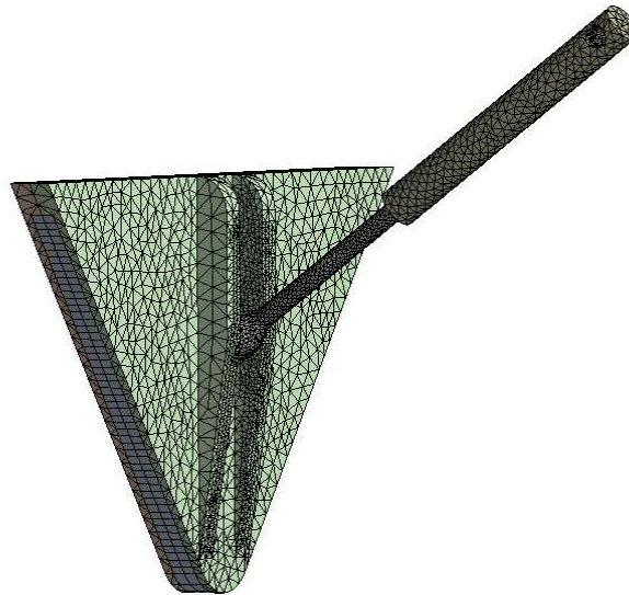
Figure 5. Finite Element Analysis Mesh
