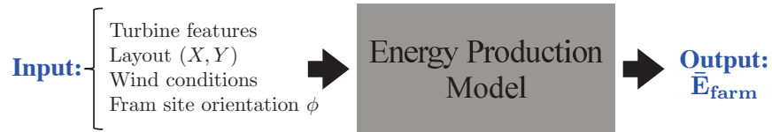
Figure 9.3: Input and output structure of the average annual energy production model
