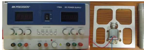
Figure 3.12 DC power supply and electric motor assembly
