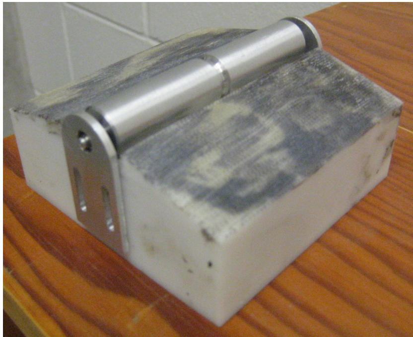
Figure 3.11 Rotating cylinder momentum injection model
