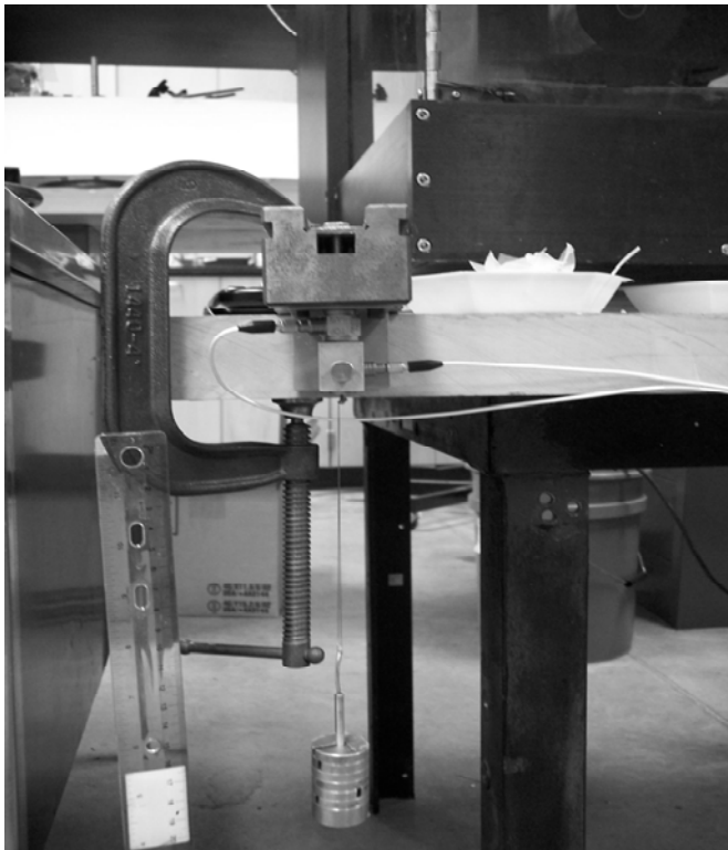
Fig. 2.7. Load cell calibration for the cross sensitivity matrix coefficients S_{zz} and S_{zx} .
