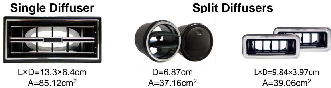
Figure 8-2 Three types of diffusers (ATDs) tested
