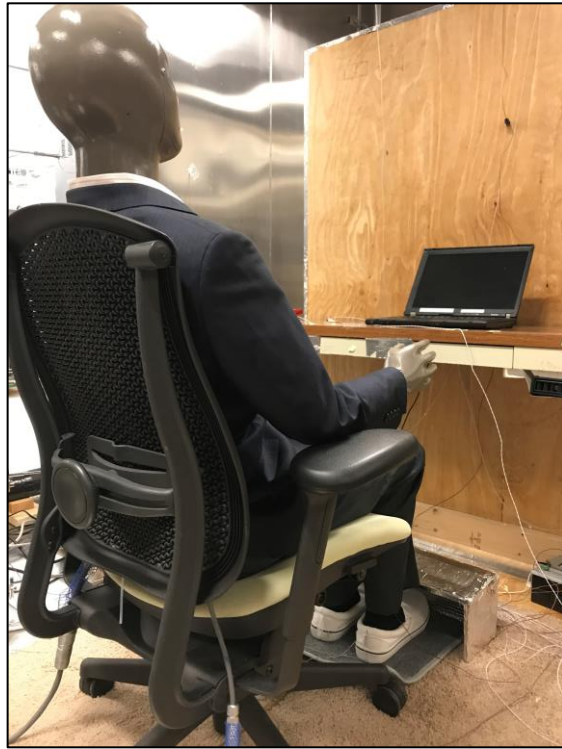
Figure 8-3 Manikin test with the heating delivering device
