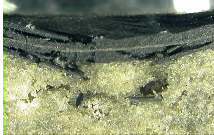
Figure 2.5 Impact damage severe enough to cause damage to the laminate
