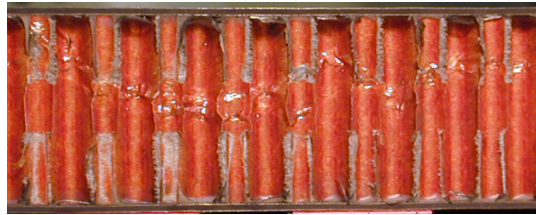
Figure 2.7 Cracked Nomex core in a honeycomb composite sandwich caused by a static load of 750 lbs using a two inch diameter puck
