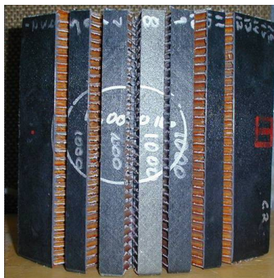
Figure 6.8 Test panel cut into strips so that the damage to the honeycomb could be examined
