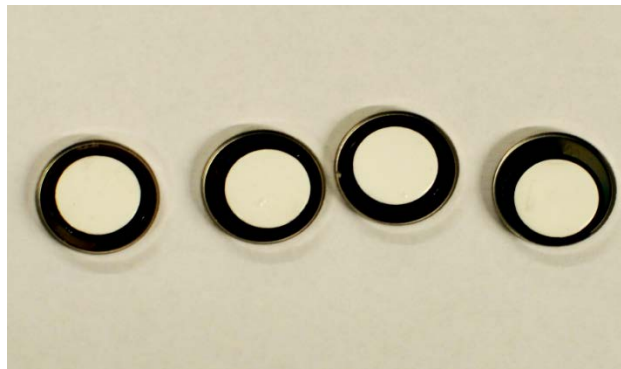
Figure 6-3 Picture of cathode chip and LATP ceramic electrolyte inside the coin cell case
