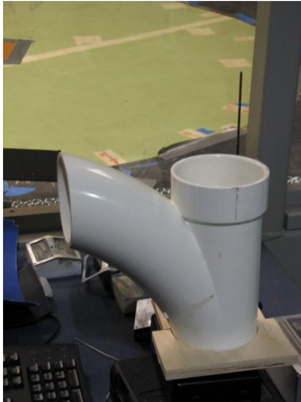
Figure A.2 Y-shaped pipe to allow forced and drawn air through throat (inverted when installed) Design modification and fabrication by J. Pierce Scarlett, photo courtesy J. Pierce Scarlett
