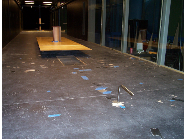
Figure 2.4 14-in. model in wind tunnel, mounted on test platform, showing pitot-static tube in front
