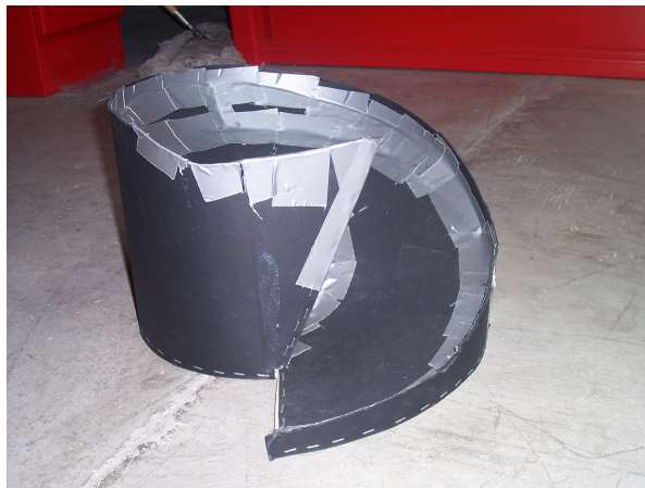
Figure A.7 Side view of ramp installation for spiral chamber floor Design modification and fabrication by J. Pierce Scarlett, photo courtesy J. Pierce Scarlett
