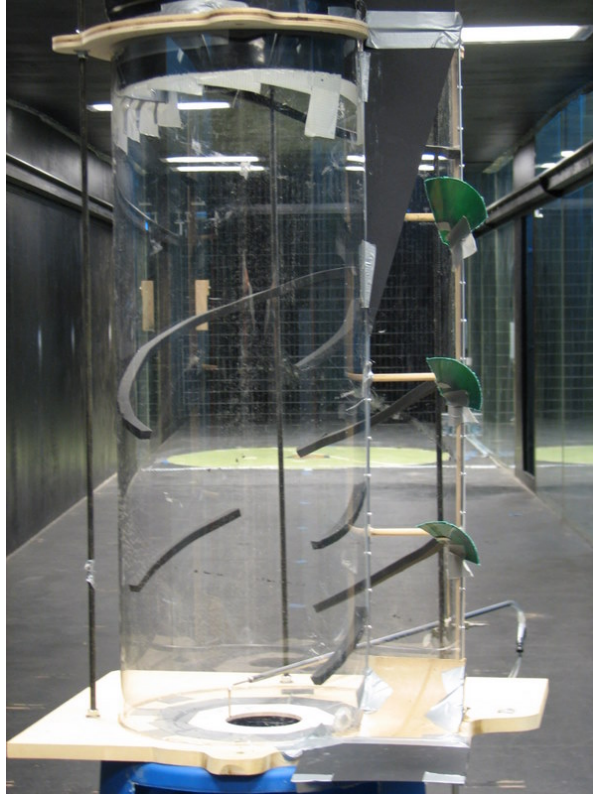
Figure A.4 Channel along spiral wall and semi-cones at spiral inlet Design modification and fabrication by J. Pierce Scarlett, photo courtesy J. Pierce Scarlett
