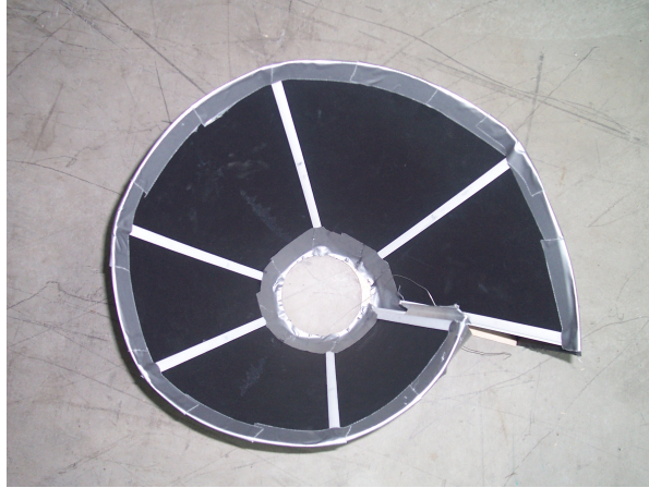
Figure A.8 Top view of inverted cone installation for spiral chamber floor Design modification and fabrication by J. Pierce Scarlett, photo courtesy J. Pierce Scarlett
