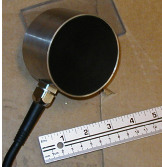
Figure 1.1: 10 MHz, segmented, annular, compound spherical, phased array transducer.
