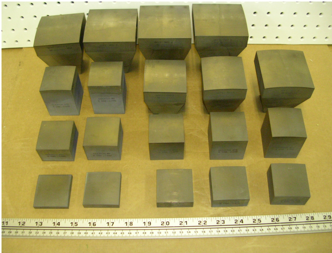
Figure 2.4: Set of curved interface calibration specimens.
