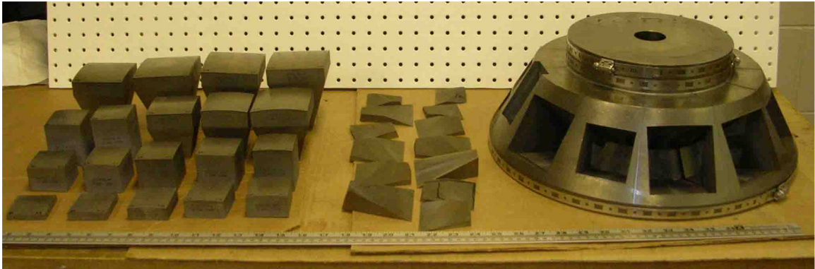
Figure 2.6: Complete HW forging disk after wire EDM, including forging coupon set, excess forging material shards, and reassembled disk as holder.
