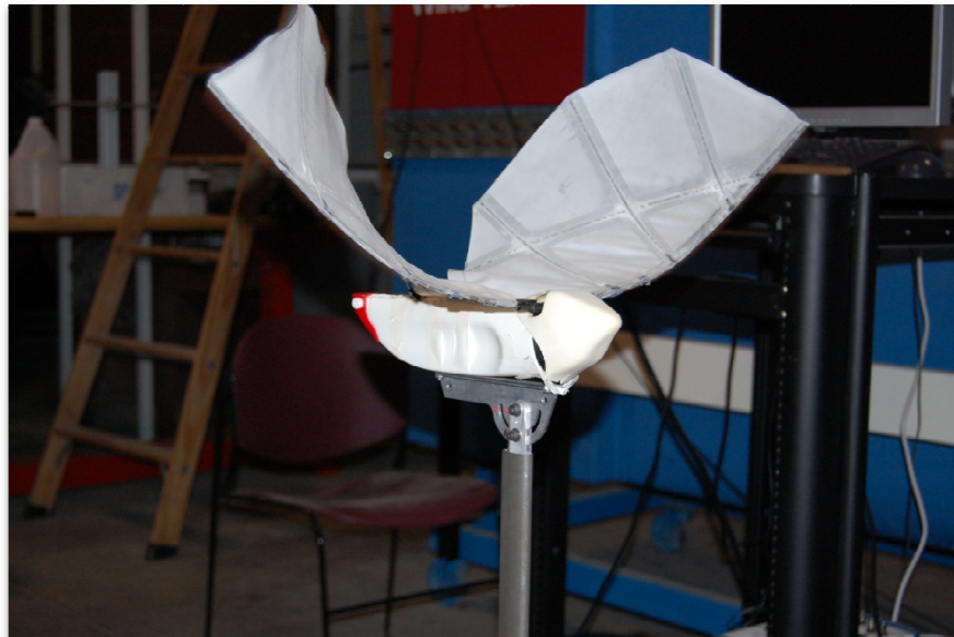
Figure 3.6. High Speed Image of Flexibility of a Latex Wing During Hovering Tests
