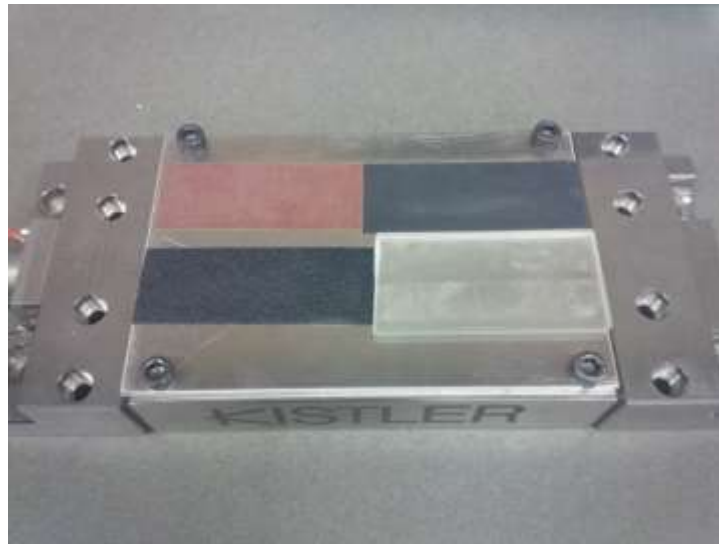
Fig. 2.1 Arrangement of the four textured samples mounted to the Kistler 9254 three-axis dynamometer: coarse texture (FEPA P100 top left), fine texture (FEPA-P2500, top right), medium texture (FEPA-P320, bottom left), fine texture (FEPA-P2500, top right), and control texture (bare acrylic, bottom right).
