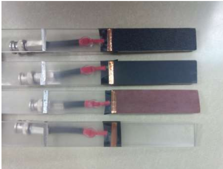
Fig. 2.2 The four texture wands for the ERP sessions; from top to bottom: Coarse, Medium, Fine, Control
