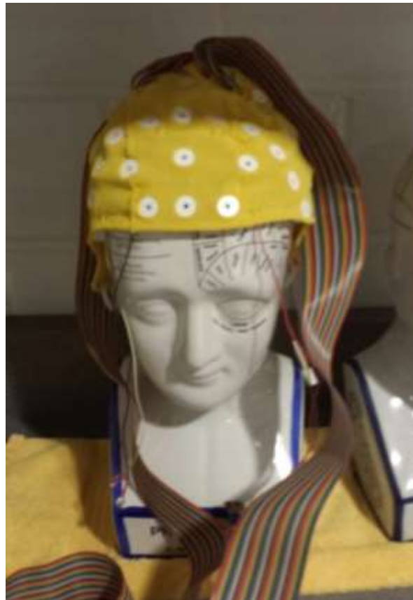
Figure 2.3. The 68-channel electroencephalogram cap used during EEG-ERP testing, where each electrode detects the scalp's electrical activity and neural response with respect to specific regions of the brain.
