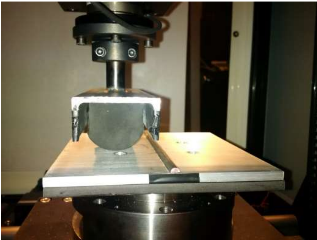
Figure 4.1. The polyurethane rod brought into contact with the counterface surface prior to a tribological test.
