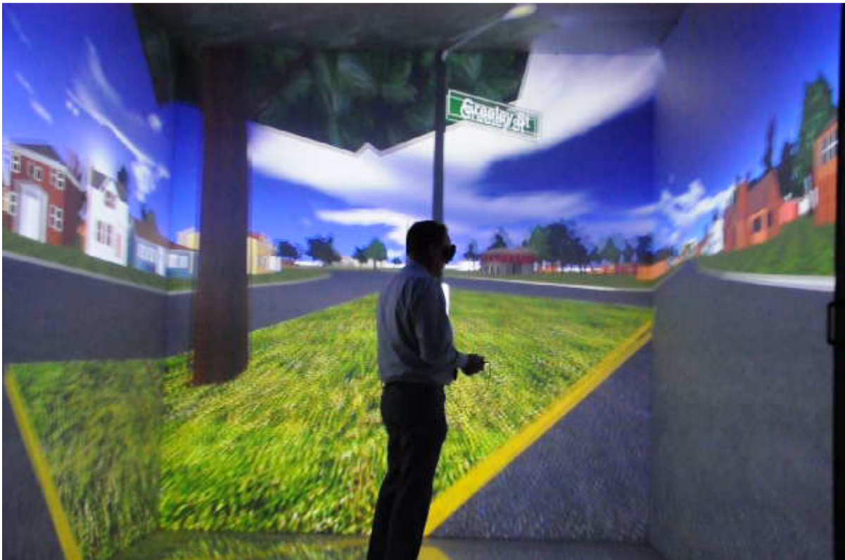
Figure 3.8 Dr. Les Miller inside the C6 immersive virtual environment. Five of the six projection walls of the environment are visible. The sixth wall is retracted to expose the participant for the shoot. A street sign of Greeley Street is in the foreground. The stereoscopic double image allows for depth perception when the user is wearing stereo glasses (pictured).
