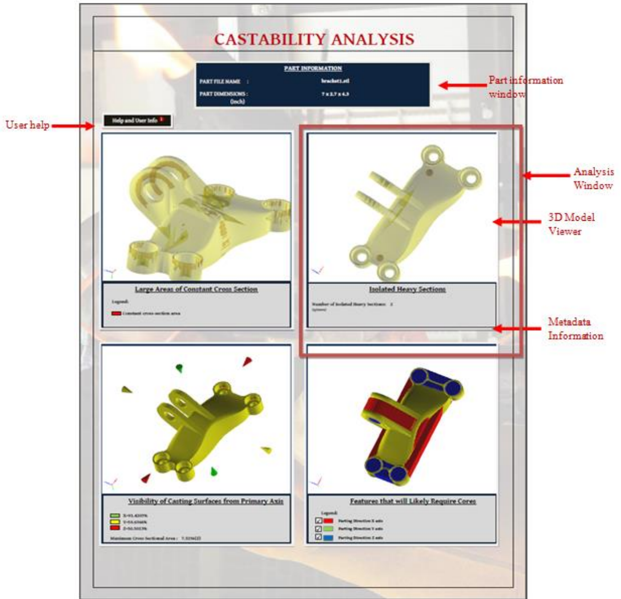
Figure 4: Three dimensional Integrated Feedback generated by CAST-ana shows multiple casting analysis results on a part design.
