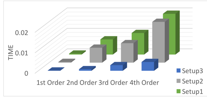
Figure 9.4 Comparison of setup1 (pure Markov model), setup2 (Markov model extended with ranking) and setup3 (Markov model extended with Situ ranking) in terms of prediction time.
