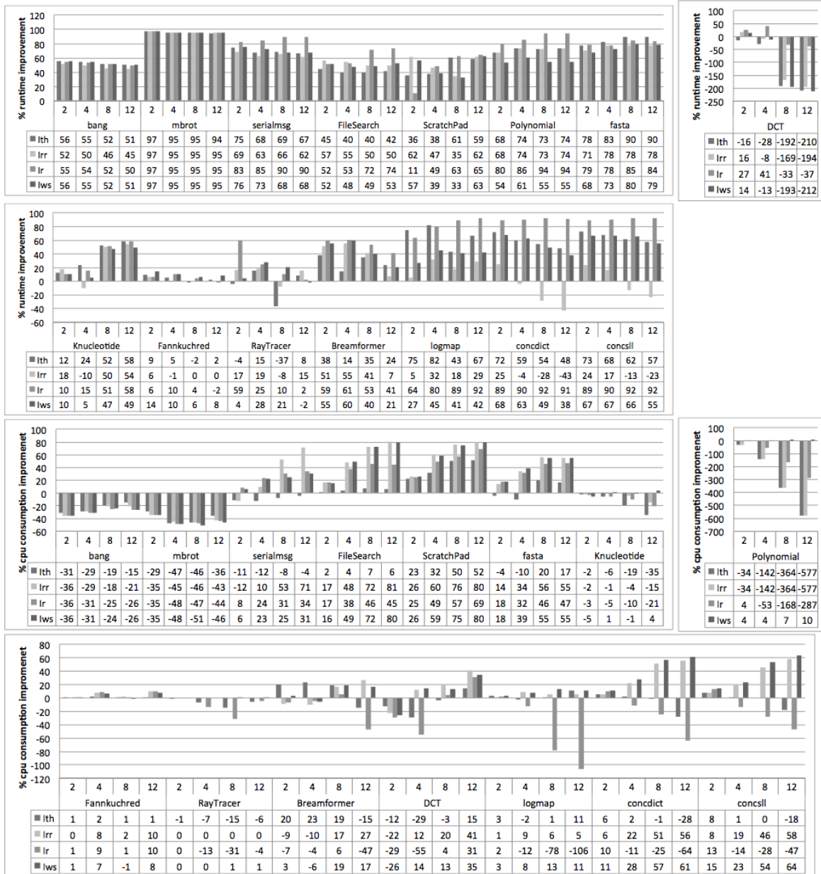
Figure 4.2 First two rows (3 charts) show % runtime improvement over default mappings, next two rows (3 charts) show % cpu consumption improvement over default mappings for fifteen benchmarks. For each benchmark there are four core settings (2, 4, 8, 12-cores) and for each core setting there are four bars (lth, Irr, Ir, lws) showing improvement over four default mappings ( thread , round-robin , random , work-stealing ). Higher bars are better.
