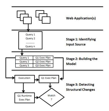
Figure 3.4: Stages involved in detecting SQLIA using Execution Plan Approach.
