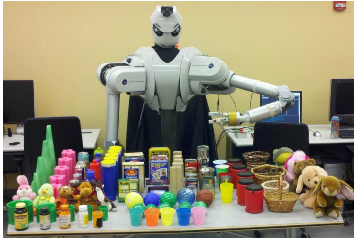
Figure 8.1 The humanoid robot used in our experiments, along with the 100 objects that it explored.
