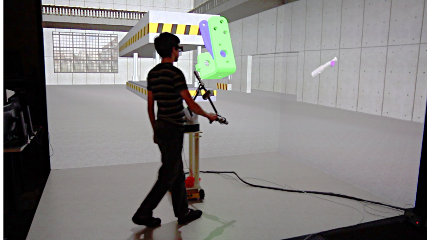
Figure 5.5: System in use simulating disassembly in METaL virtual reality system with Haption Virtuose
