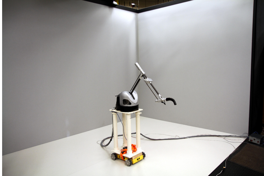
Figure 5.1: Haption Virtuoso on Mobile Robot in METaL Virtual Reality System
