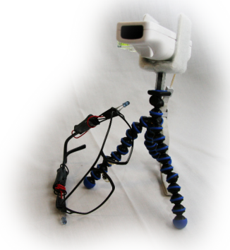
Figure 2.3: Wii Remote, tripod mount, and trackable glasses
