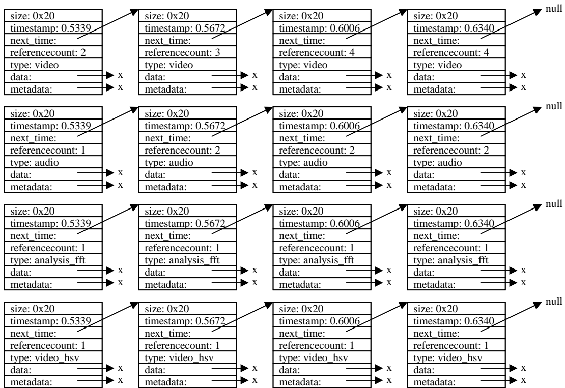
Figure 3.1: Organization of the packet system in the middleware. Packets are stored in a linked list, allowing both dynamic allocation and traversal to temporally close packets of similar type. Each type of data (e.g. VIDEO) is stored in its own linked list. The system maintains all the packets of the system through an array of linked lists (storing both the head and tail of each list), which each array index corresponding to a unique data type.
