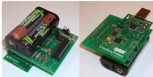
Figure 3.9 TelosB power meter kit used in LB-MAC. The working power consumption of this kit is 2.4\mu\text{W} which is small compared to radio power consumption.
