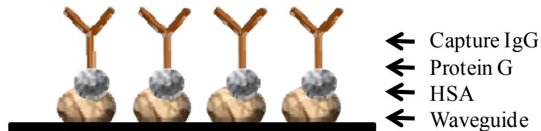
FIGURE 3. Orientation of Antibody on a HSA-PG Coated Waveguide Surface
