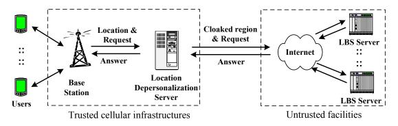
Figure 3.1 System architecture
