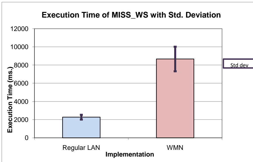
Figure 441 - MISS_WS in a regular network and a WMN with their standard deviation
