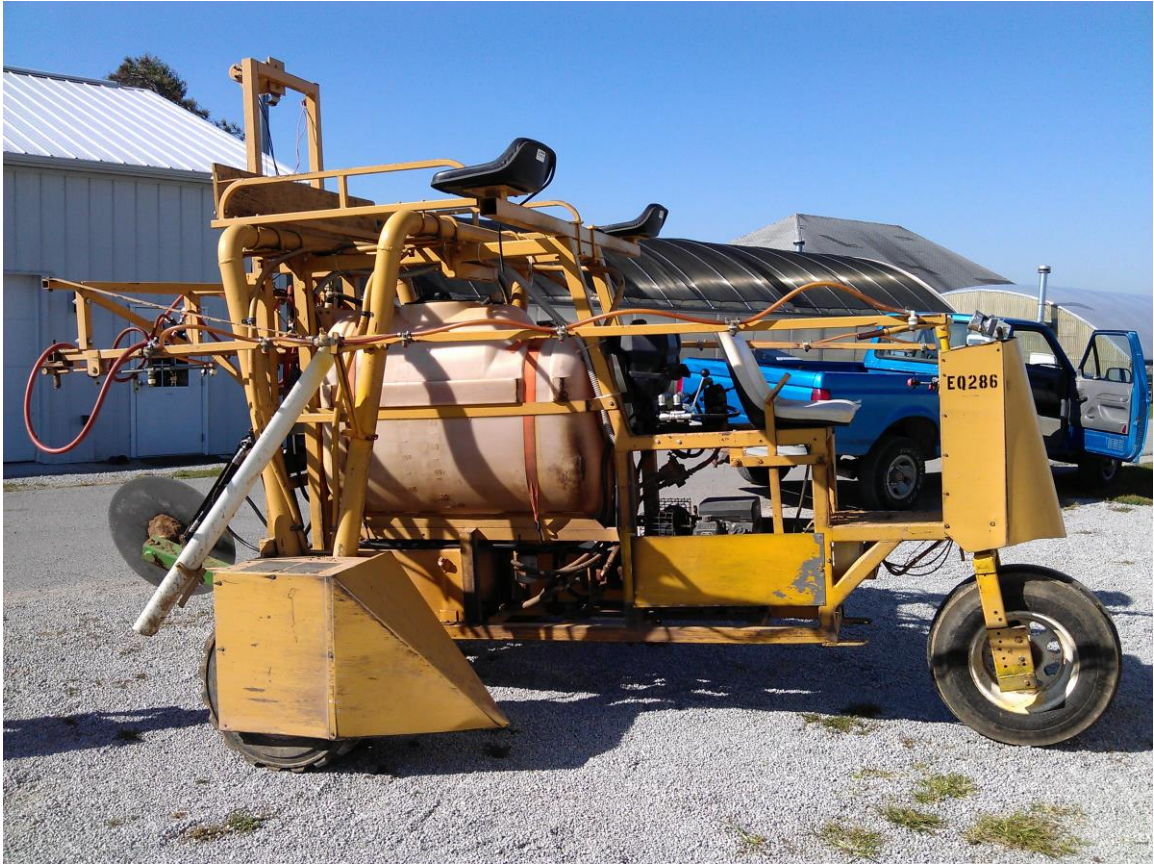
Figure 5-1 - Tri-wheeled tobacco sprayer used in Phase 3
