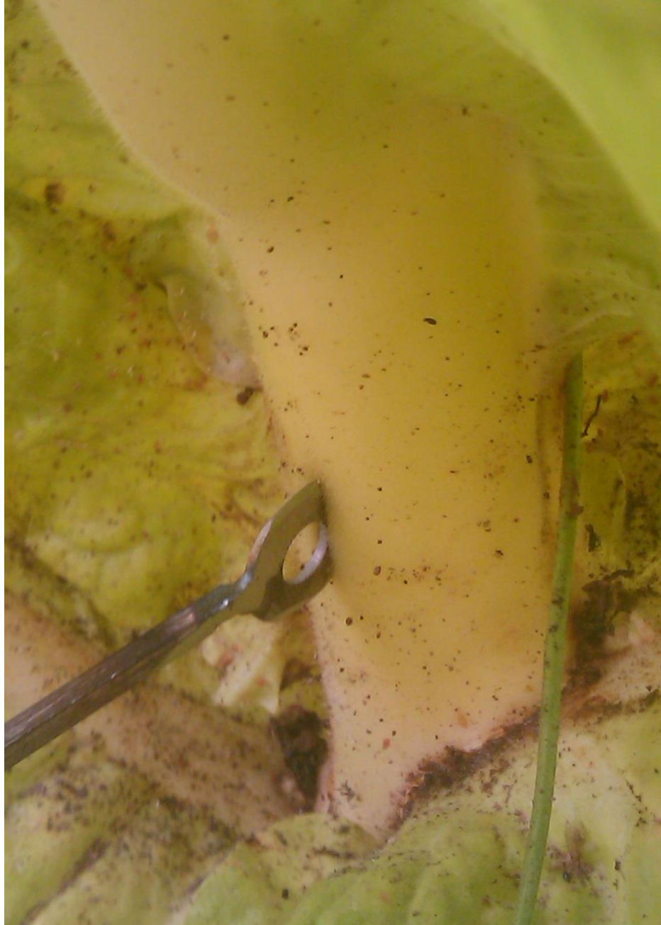
Figure 3-1 - A custom drill bit fabricated to bore the pith out of a tobacco stalk without damaging the structural integrity
