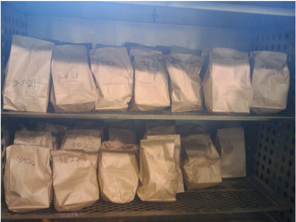
Figure 3-4 - Paper bags in the drying oven, each with a tobacco leaf inside
