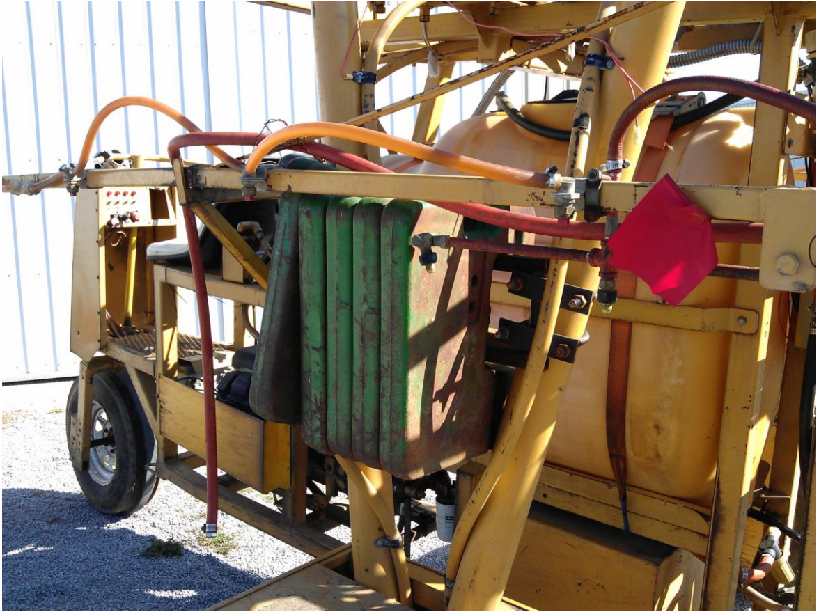
Figure 5-3 - Ballasts added to one side of the sprayer to combat uneven loading
