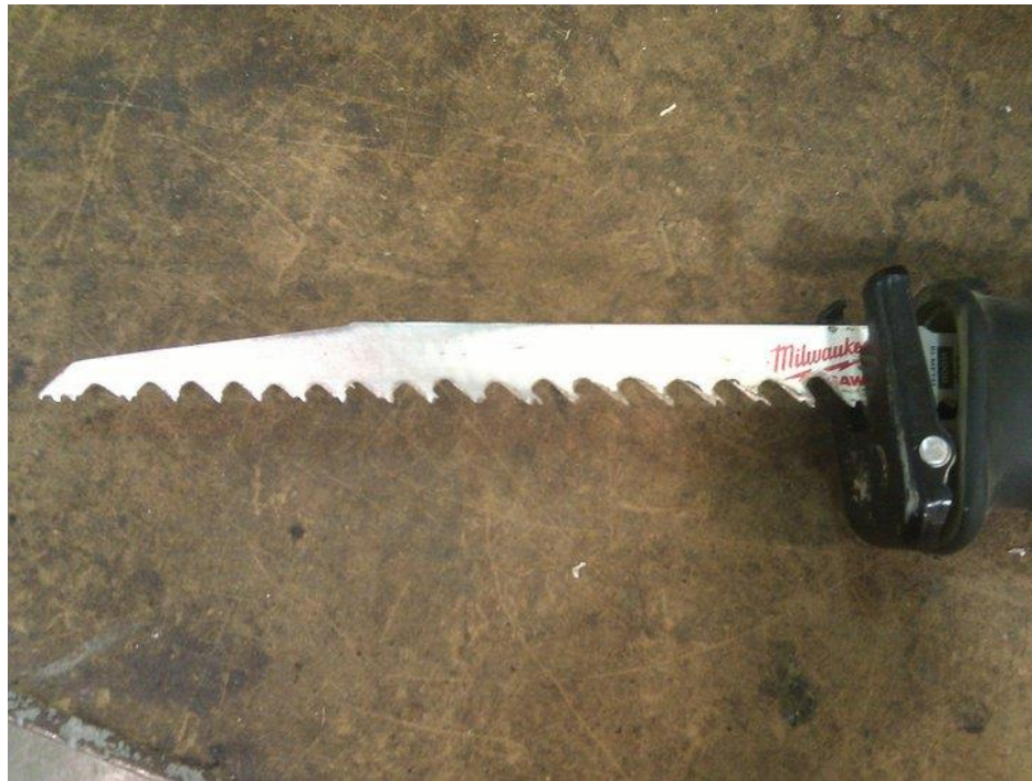
Figure 4-1 - modified reciprocating saw blade
