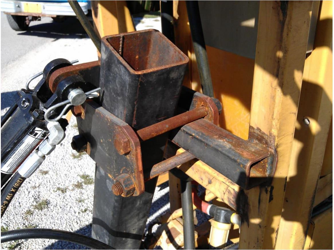
Figure 5-7 - Coulter disc implement affixed to the sprayer via mounting plates
