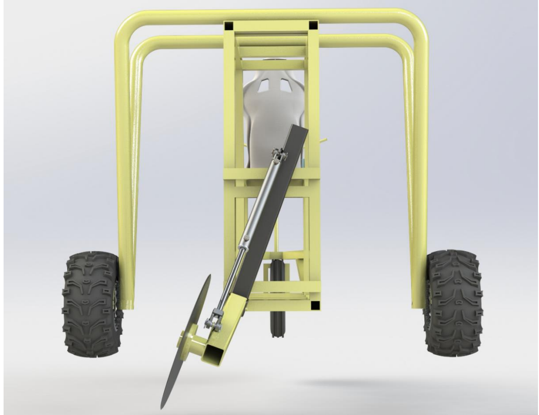
Figure 5-4 - CAD model of the possible interaction between the extended coulter arm and the soil
