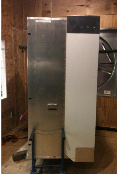
Figure 3-21 – Extension positioned on 54" FANS unit
