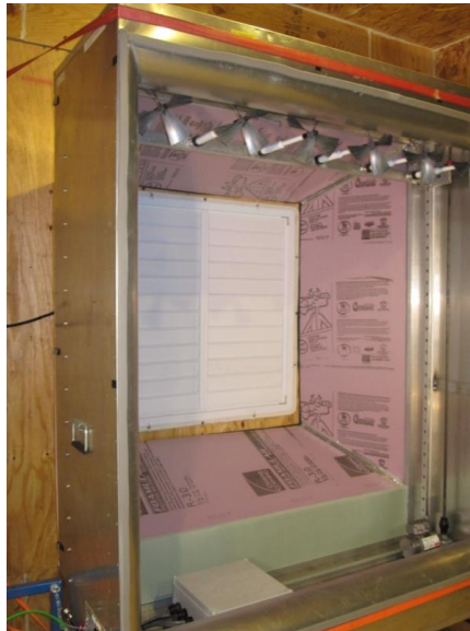
Figure 4-10 – Fan testing setup; treatment 36_54_60I
