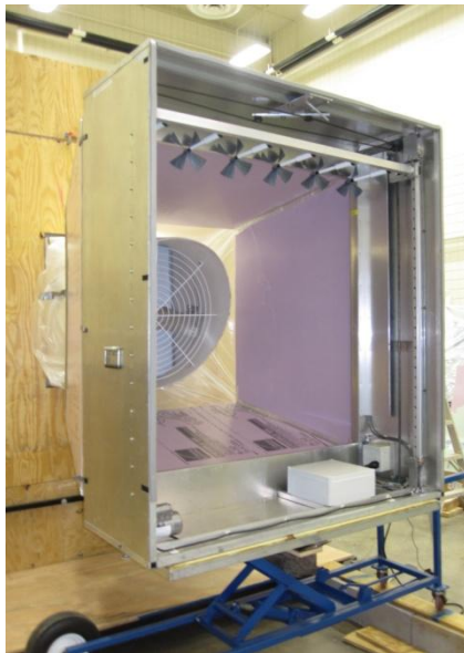
Figure 4-12 – Fan testing setup; treatment 36_54_30D
