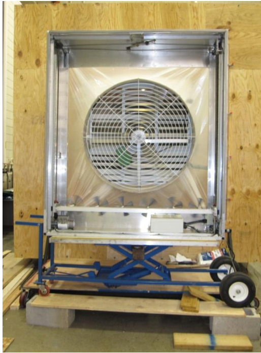
Figure 4-24 – Fan testing setup; treatment 48_54_ND
