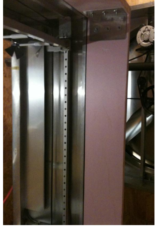
Figure 3-21 – Extension positioned on 54" FANS unit
