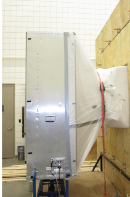
Figure 4-11 – Fan Testing setup; Treatment 36_54_D
