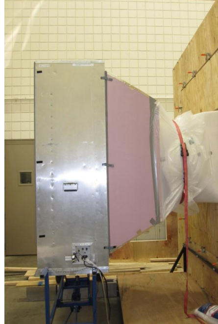
Figure 4-13 – Fan testing setup; treatment 36_54_45D
