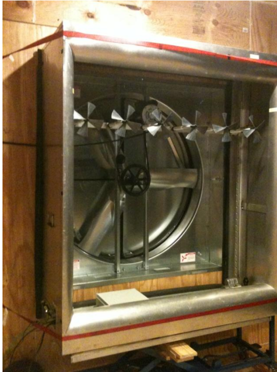
Figure 4-25 – Fan testing setup; treatment 54_54_I
