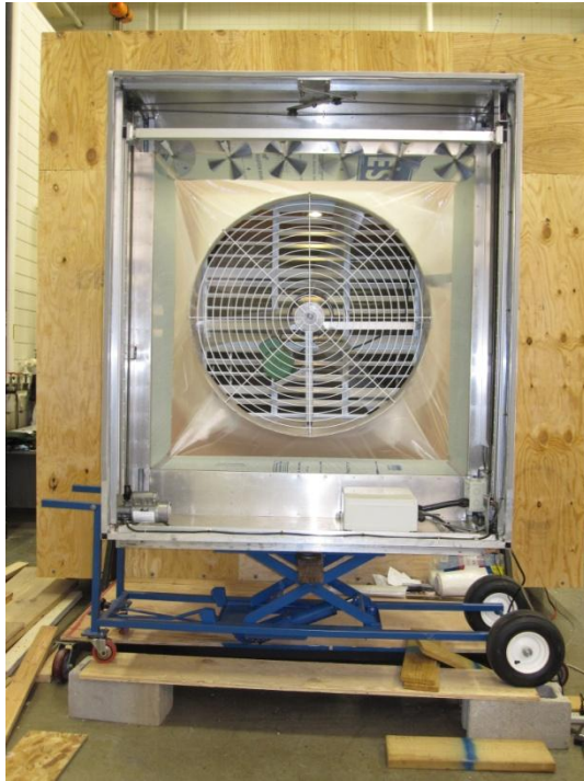
Figure 4-22 – Fan testing setup; treatment 48_54_45D
