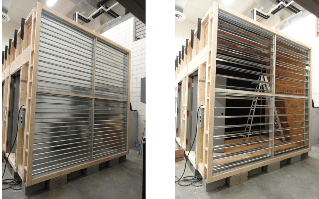
Figure 3-9 – WINTAC: Inlet wall (closed and opened)
