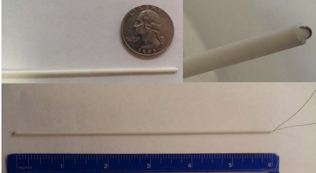
Figure 5.3.2 Heating wire coated with silicone paste and inserted through ceramic tube. Rubber silicone glue was applied at the terminal end of the probe to protect the heating wire loop.
