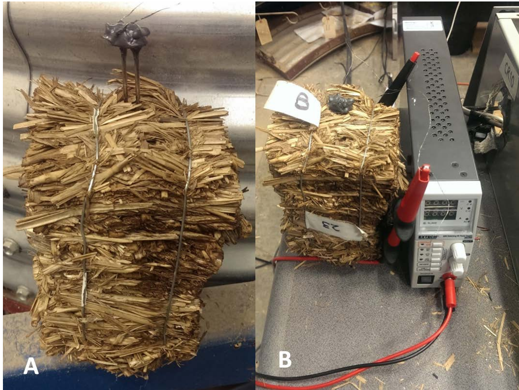
Figure 5.3.7 Experimental testing of the dual thermal probe in miniature bales of switchgrass. A) Insertion of the dual probe into a bale to measure the lateral direction; and B) connection of the voltage source to the heating wire.
