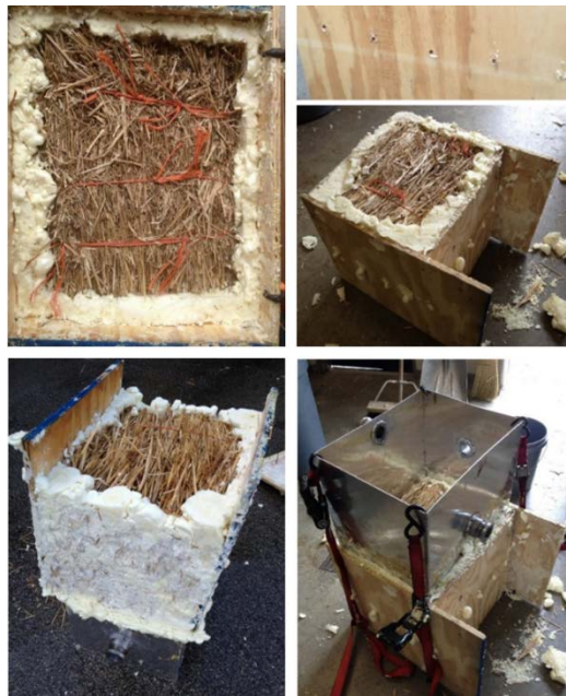
Figure 5.1.2 Bale fitted in plywood frame with spray insulation foam preventing boundary flow.
