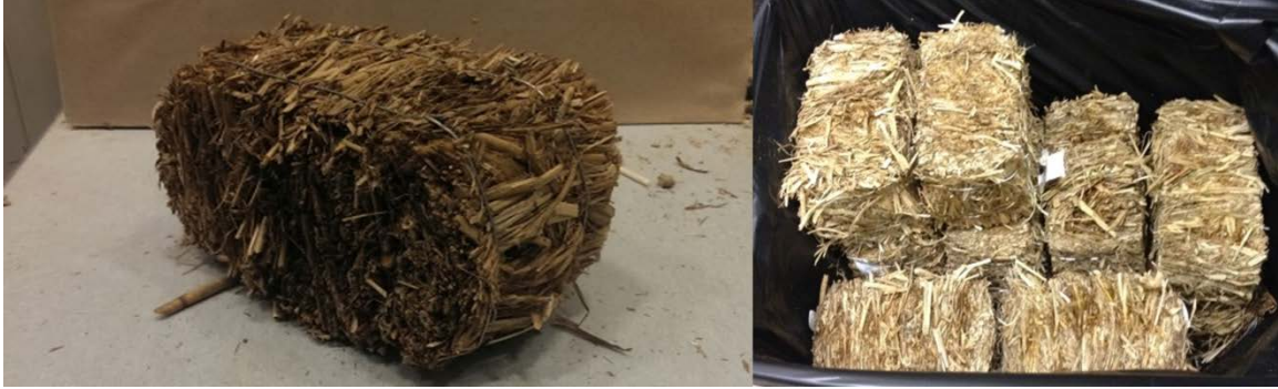
Figure 5.2.2. Flake compaction to form miniature bales ( 38 \times 46 \times 94 \text{ cm}^3 ) using a newly fabricated bale chamber.
