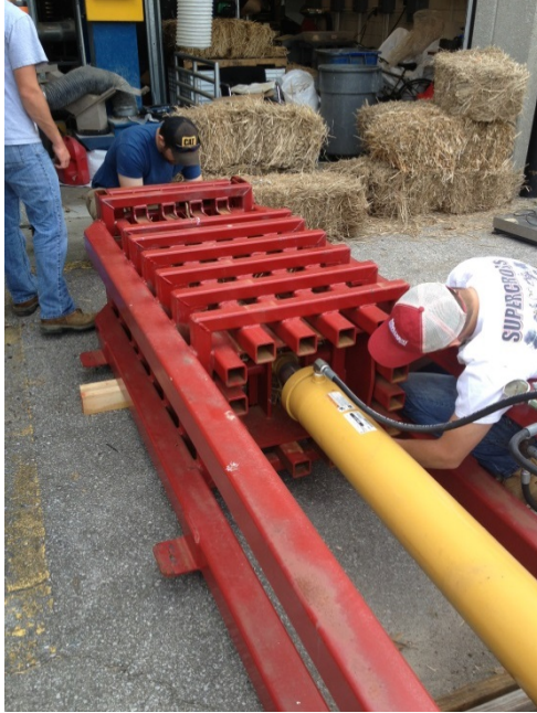
Figure 5.1.1 Compression of bales in the transverse direction using a 20.68 MPa (3000 psi) hydraulic press.
