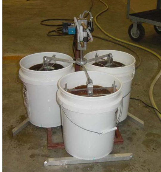
Figure A.7: Pneumatic Wet Sieving Device Used in Eroded Particle Size Analysis
