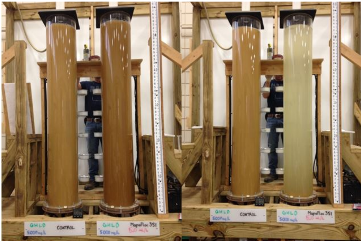
Figure 3.11: Column Comparison at 5,000 mg/L Initial Concentration at Time=0 min (left) and Time=5 min (right)
