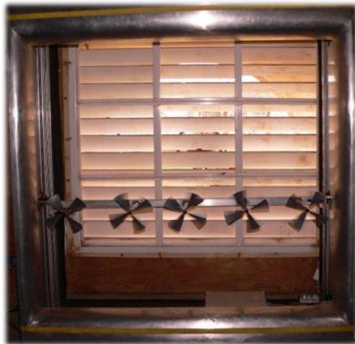
Figure 3.31. FANS unit (serial number: 48-0023), anemometer propellers.
