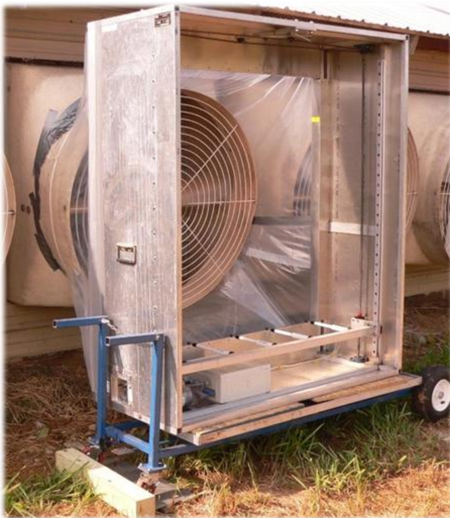
Figure 3.17. FANS unit (serial number: 48-0023) near the discharge side of the test fan, outside setup.
