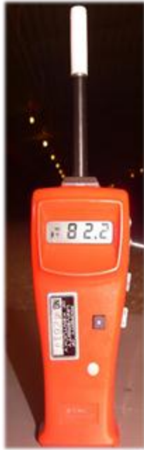
Figure 3.28. Temperature/Humidity sensor - Rotronic Hygroskop GT-1 Rotronic Instrument Corp. 135 Engineers Rd Suite 150 Hauppauge NY,11788
