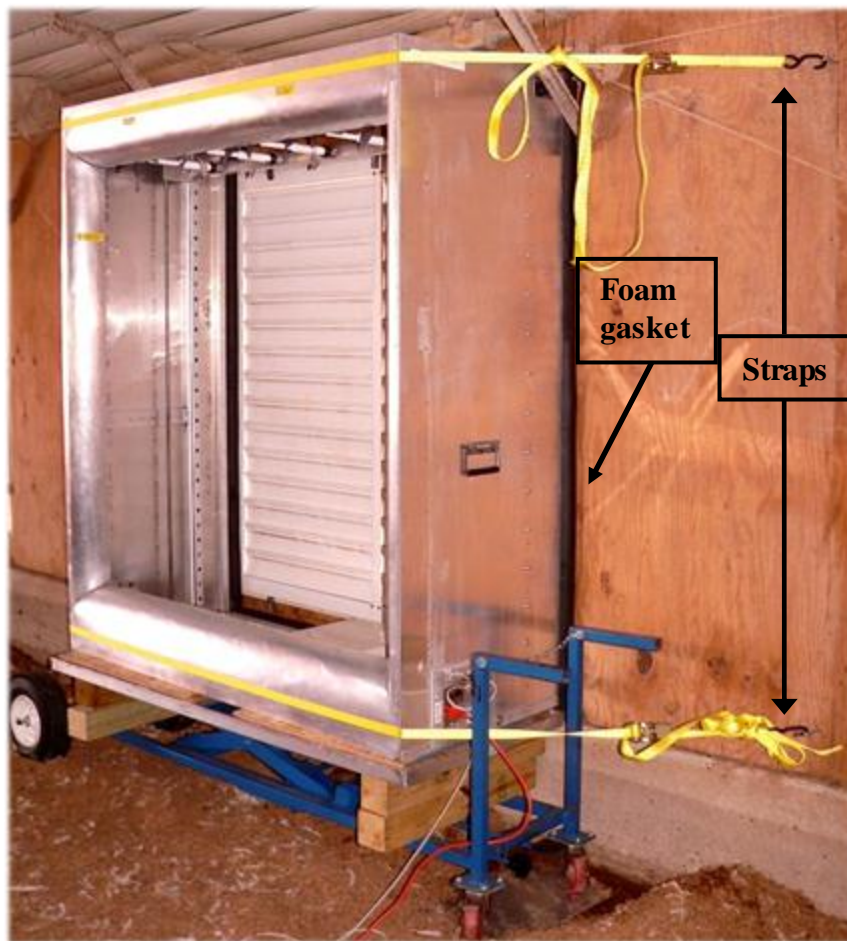
Figure 3.16. FANS unit (serial number: 48-0023) placement next to the intake side of the test fan, cart, foam gasket and straps.
