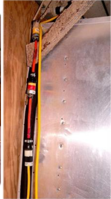
Figure 3.24. Power cords. Arrow 1 indicates the extension cord between the power supply and power meter. Arrow 2 indicates the extension power cord between the power meter and the fan.
