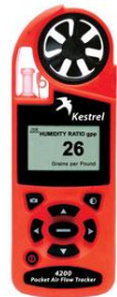
Figure 3.26. Kestrel 4200, Pocket Air Flow Tracker (operational range of 0 - 99.999,00 \text{ m}^3 \text{ h}^{-1} \pm 3.0\% )
