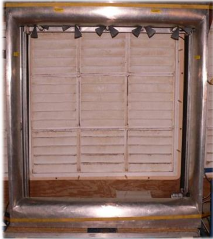
Figure 2.5. Front view of the 1.22 m (48 in) FANS unit set up next to the intake side of an exhaust fan.
