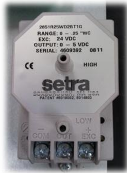
Figure 3.19. Differential Pressure Transducer (Setra Systems Model 265, series 0811)
