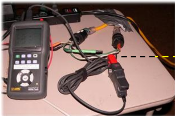
Figure 3.25. Setup of AEMC PowerPad Jr, Model 8230. The arrow indicates the connector cord with separated wires for clamp-on measurements and spliced connections for voltage probes.
