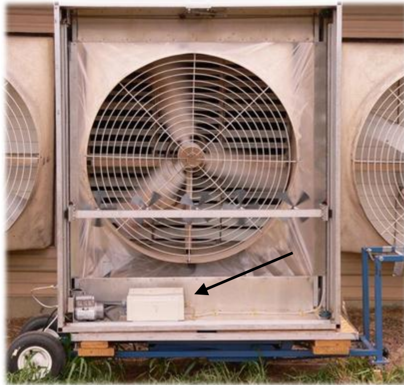
Figure 3.18. FANS unit (serial number: 48-0023) outside setup, static pressure sensor.
